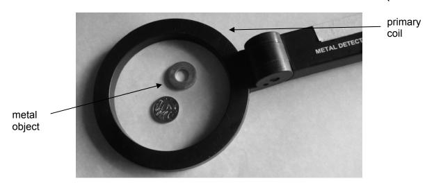
Above is a picture of a metal detector and a metal object. A ten cent coin has been added to give a sense of scale. The detector consists of a DC battery connected to a primary coil. There is a secondary coil connected to a buzzer that makes a sound when the primary coil moves over a metal object.
