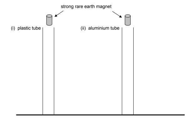
The magnet falling through the plastic tube travelled much faster than the magnet falling through the aluminium tube.
