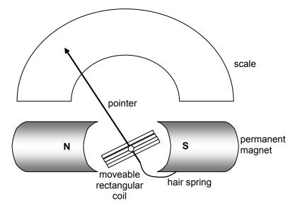
(a) When a current flows in the rectangular coil, a force is produced on each side of the coil that interacts with the magnetic field. Explain the reason for this force and comment on its direction. You must draw a diagram to illustrate your explanation. (3 marks)
