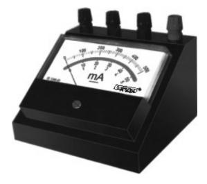
The coil inside the meter is not designed to take large currents. If the ammeter is required to measure a maximum reading of 1.50 A, an additional resistor called a *shunt* has to be added as shown below. The meter has a coil resistance of 5.00  $\Omega$ . This arrangement is shown here:
