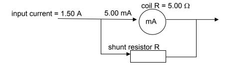
Find the value of the shunt resistor R.
